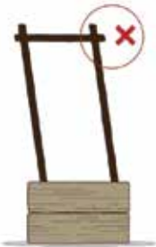
1. NOT LEANING OR UNSTABLE
